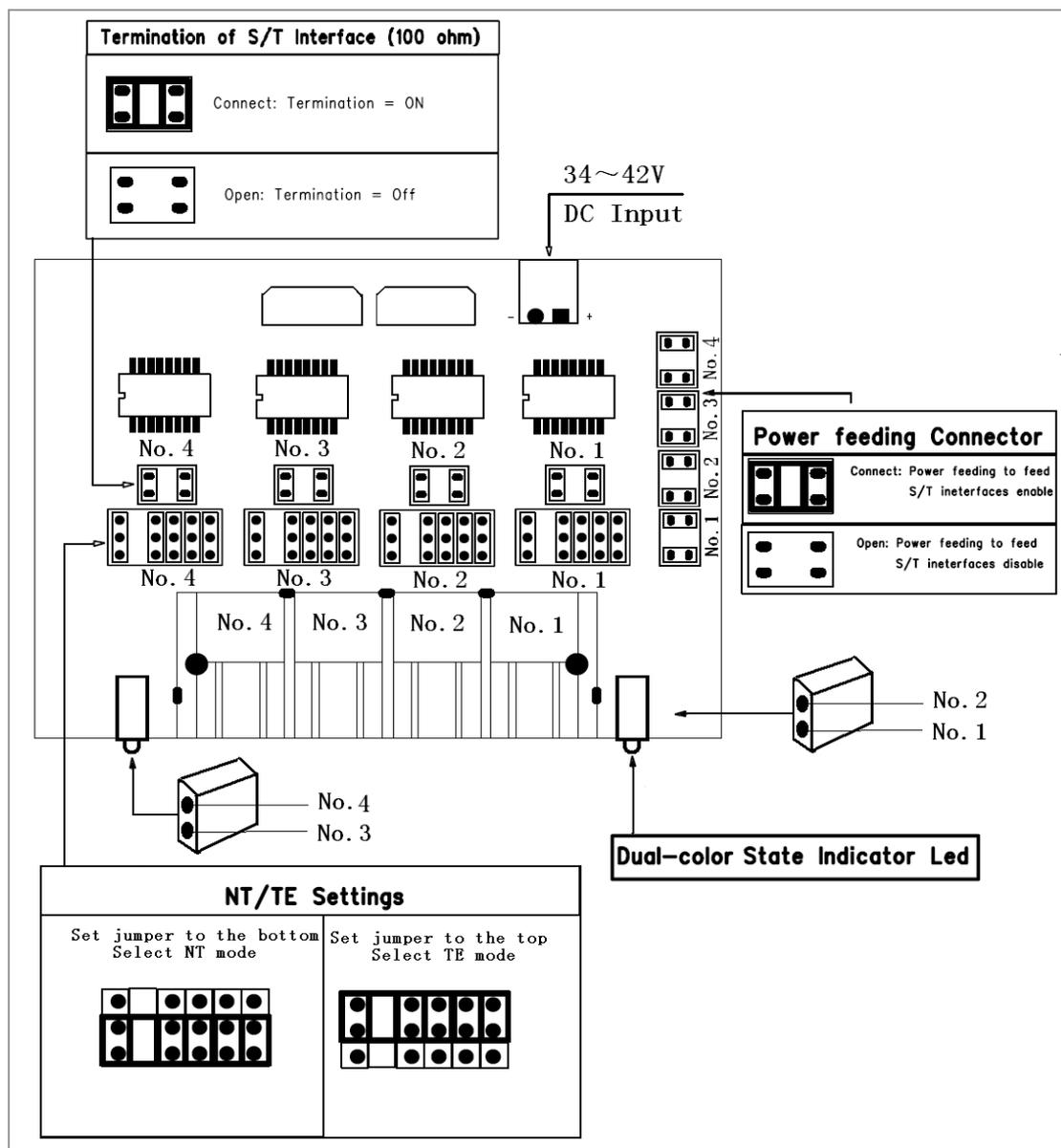
Figure 5 Jumper Setting
