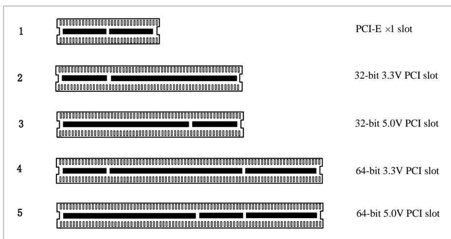
Figure3 PCI-E and PCI slots
